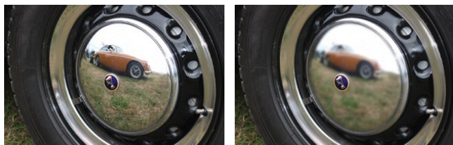
Example of a coated and polished surface without and with Reflected Haze
